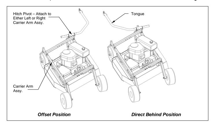
Figure 5: Assembly of the Tongue and Hitch Pivot
